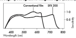
SFX 200 has a peak red sensitivity at 720nm and extended red sensitivity up to 740nm.
