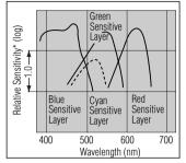
Process : C-41/CN-16 Densitometry : Status M : 1.0 above minimum density Density \*Sensitivity equals the reciprocal of the exposure (J/cm<sup>2</sup>) required to produce a specified density
