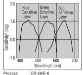
Densitometry : Status A Density : 1.0 above minimum density \*Sensitivity equals the reciprocal of the exposure (J/cm<sup>2</sup>) required to produce a specified density
