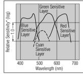
Process : C-41/CN-16 Densitometry : Status M Density : 1.0 above minimum density. 'Sensitivity equals the reciprocal of the exposure (J/cm²) required to produce a specified density
