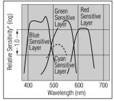
Process : C-41/CN-16 Densitometry : Status M Density : 1.0 above minimum density \*Sensitivity equals the reciprocal of the exposure (J/cm<sup>2</sup>) required to produce a specified density
