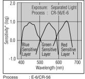
Densitometry : Status A : 1.0 above D-min Density \*Sensitivity equals the reciprocal of the exposure (J/cm<sup>2</sup>) required to produce a specified density
