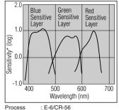
Densitometry : Status A Density : 1.0 above minimum density \*Sensitivity equals the reciprocal of the exposure
