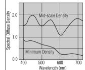
Process : C-41/CN-16 Densitometry : Status M Densitv : 1.0 above minimum density \*Sensitivity equals the reciprocal of the exposure (J/cm<sup>2</sup>) required to produce a specified density
