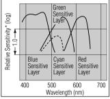
Process C-41/CN-16 Densitometry : Status M Densitv : 1.0 above minimum density \*Sensitivity equals the reciprocal of the exposure (J/cm<sup>2</sup>) required to produce a specified density
