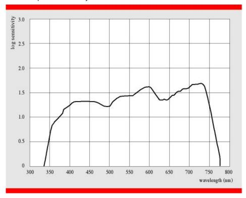
Sensitivity is reciprocal of the exposure (mJ/m²) required to produce a diffuse density of 1.0 above fog. Processed in Gevatone 66, G 74 c developer at 30 °C for 42 seconds.
