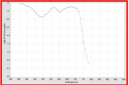
Sensitivity is reciprocal of the exposure  $(mJ/m^2)$  required to produce a diffuse density of 0.3 above fog. Processed in Gevatone 66, G 74 c developer at 30°C for 42 seconds.
